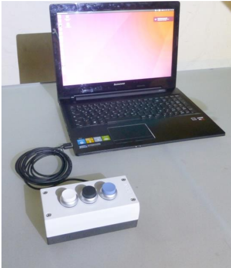
Screen 49: Individual programming for each button in the PBL series
