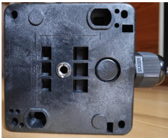
Screen 48: bottom view of pushbutton with mounting holes
