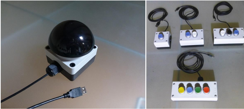
Screen 1: USB pushbutton (left) and USB pushboxes (right)
