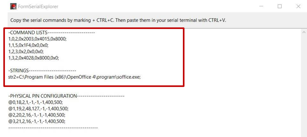
Screen 20: Correct command list and string in the FormSerialExplorer (via Show serial cmds )
